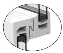
Interlocking meeting rails with optional weatherstrip provides additional protection against air infiltration between sash.
